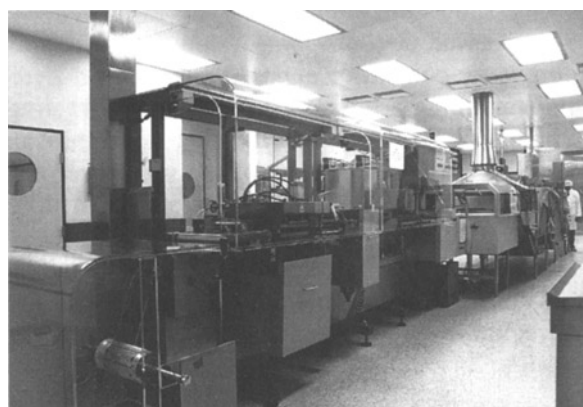
Figure 5. Form-fill blister-pack machine.
